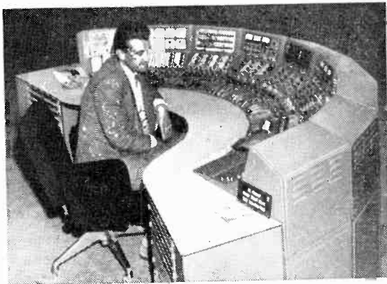
Console of the 34-channel sound mixer manufactured by Pye for the E1stree Studios of Associated Television. In addition to providing mixing facilities for studio microphones it also provides echo effects and talk-back facilities.
